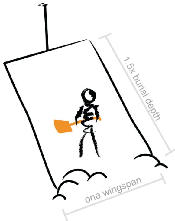
Figure 6. In burials deeper than one meter, it is important to begin the excavation downhill about 1.5 times the burial depth (in typical debris piles). This prevents the hole from becoming too narrow as you approach the buried victim. Our field experience shows that once shovelers begin digging, it is counter-intuitive for them to expand the hole away from the victim. Therefore, the excavation should start from below and work inward to the victim.
